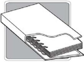
**Cased In** – Standard wire-o pasted into a hard case with all the advantages of opening.
