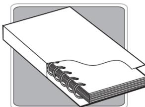
**Half Canadian** – (Back Cover Bind) – The partially hidden wire-o is exposed on the back cover. Flat spine allows for easy identification.
