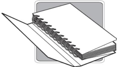
**Reverse Binding** – Allows for an expandable inside cover where a large spread image is important. The binding is hidden and the spine is flat. Back flap can be pasted down or left free.
