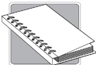
**Full Canadian (Square Back)** – The partially hidden wire-o is exposed on the front and backcover. Flat spine allows for easy identification.
